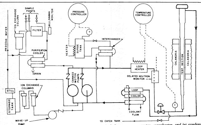
The main loop circuit in this simplified flow sheet of a typical loop is indicated by the heavy line. Specific loops are, of course, more complex. The X-4 loop, for example,
